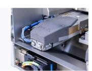
The seeds are cleaned with air streams to remove dust and debris, then transferred to a vibrating plate for alignment. When on the plate, each seed is photographed, enabling advanced imaging software to count and analyze their quality and characteristics.
