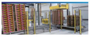
Viscon's palletising and de-palletising solutions are able to process a diverse variety of: boxes, crates, various types of trays, and virtually any product of a rectangular design. These units can be integrated with pallet strapping and/or wrapping units as well. Viscon supplies several unique buffer systems which enable many types (sizes/grades) of products to be processed through one palletising unit.
